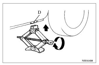
6. Rotate the jack by hand until the flange portion (D) fits in the groove at the top of the jack.
